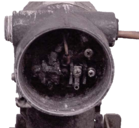
Figure 12: Corrosion of terminal arrangement in a transmitter housing due to water penetration.
